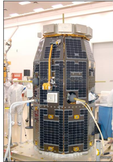
Figure 7. Photograph of the C/NOFS satellite with experiments installed at General Dynamics prior to delivery to the launch vehicle.
