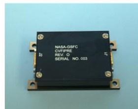
Figure 23. Photograph of the cylinder pre-amp box (left) and its circuit board (right) which was at the base of the booms that accepted the cylindrical sensor input.
