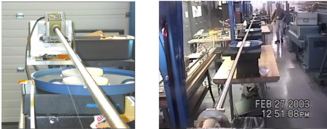
Figure 17. Boom element testing on water table in horizontal direction.
