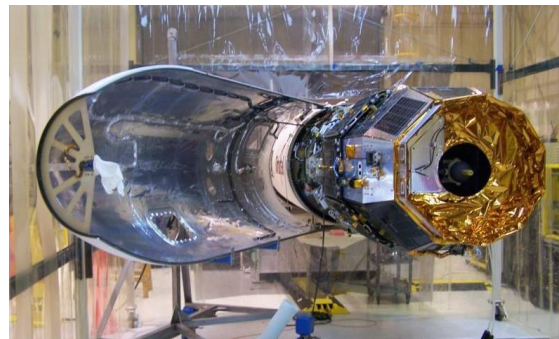
Figure 3. Photograph of the C/NOFS satellite inside the Pegasus fairing.
