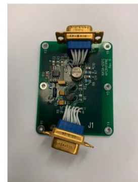
Figure 23. Photograph of the cylinder pre-amp box (left) and its circuit board (right) which was at the base of the booms that accepted the cylindrical sensor input.
